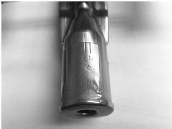
Burner Set at LP
